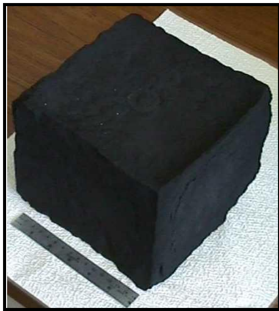
Figure 3: Manufactured Block of Reticle Carbon (Block Shown Has 1400 m 2 /g)
