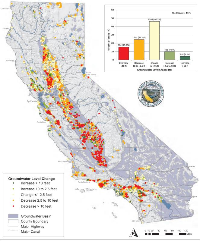
\*Groundwater level change determined from water level measurements in wells. Map and chart based on available data from the DWR Water Data Library as of 07/15/2015. Document Name: S2015\_S2014\_DM\_20150717 Updated: 07/18/2015 Data subject to change without notice.
