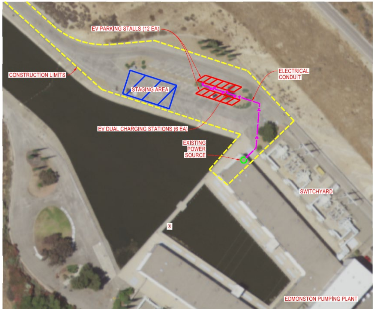
Figure 2-2. Edmonston Pumping Plant Preliminary Layout
