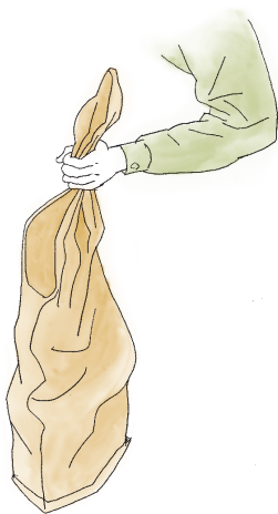
Figure 12A: Sandbag filled 1/4 to 1/3 full
