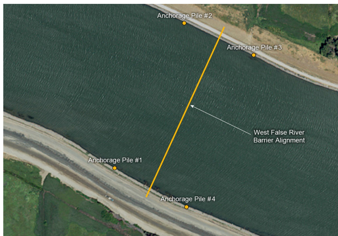
Figure 3-14 Location of Navigational Aid Ball Float Anchorage Piles
