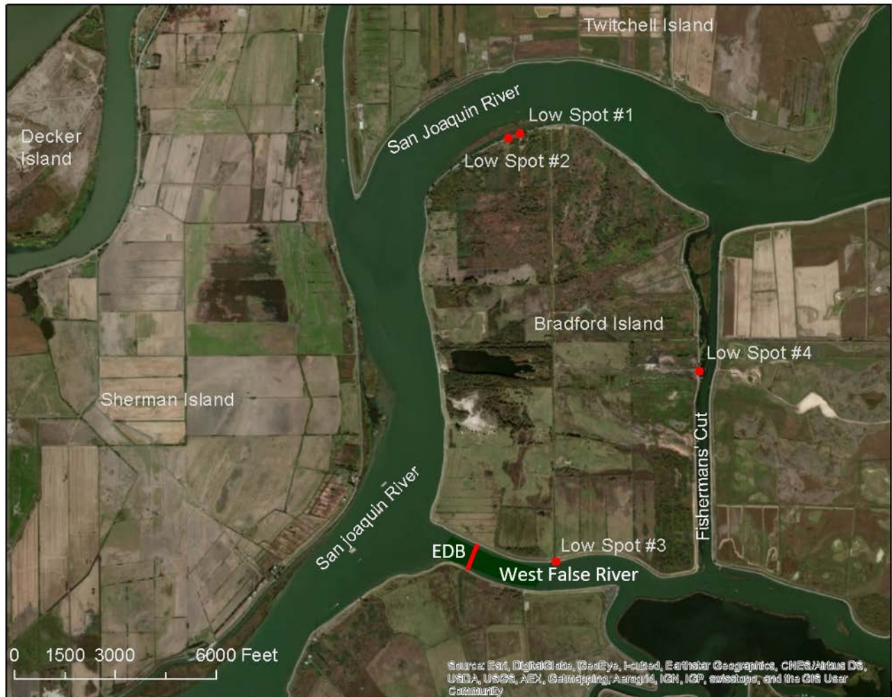
Figure 4-12 Low/Vulnerable Sections of Levees Identified by DWR and RD 2059
