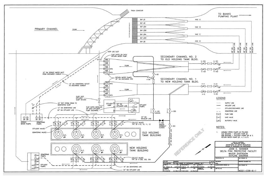
*Figure 1*- *Schematic of the John E. Skinner Delta Fish Protective Facility.* The "Old Holding Tank Building" is also referred to as HTB #1, and the "New Holding Tank Building" is also referred to as HTB #2.
