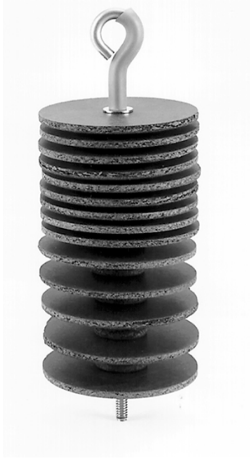
Figure 15. Hester Dendy artificial substrates for sampling benthic algae and invertebrates. The plates are three inches in diameter and easily fit into a quart Mason jar for ease of preservation for later analysis in the lab.
