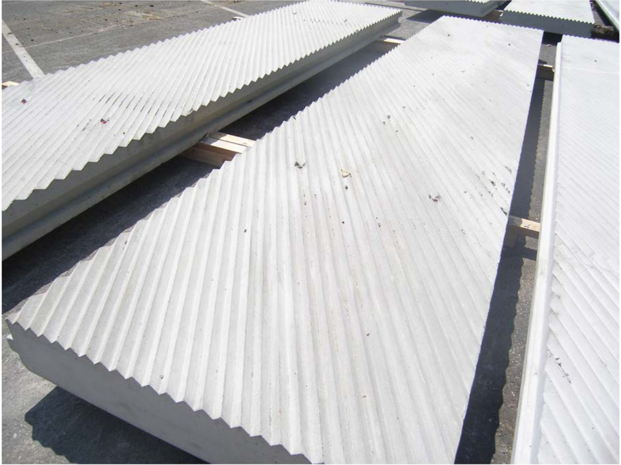
Figure 11. . Artificial sampling substrate modules of precast concrete to permit seine sampling within Dutch Slough in a manner similar to that performed by the Juvenile Fish Monitoring Programs of the USFWS. These materials are usually used to construct boat ramps
