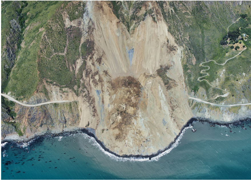
On May 20, 2017, more than 2 million cubic meters of rock and dirt collapsed down the steep slopes at Mud Creek on California's Big Sur coast. A pile of rubble almost a third of a mile wide buried California State Highway 1 more than 65 feet deep and added about 13 acres of new land to the coast. Photo: USGS, May 27, 2017
