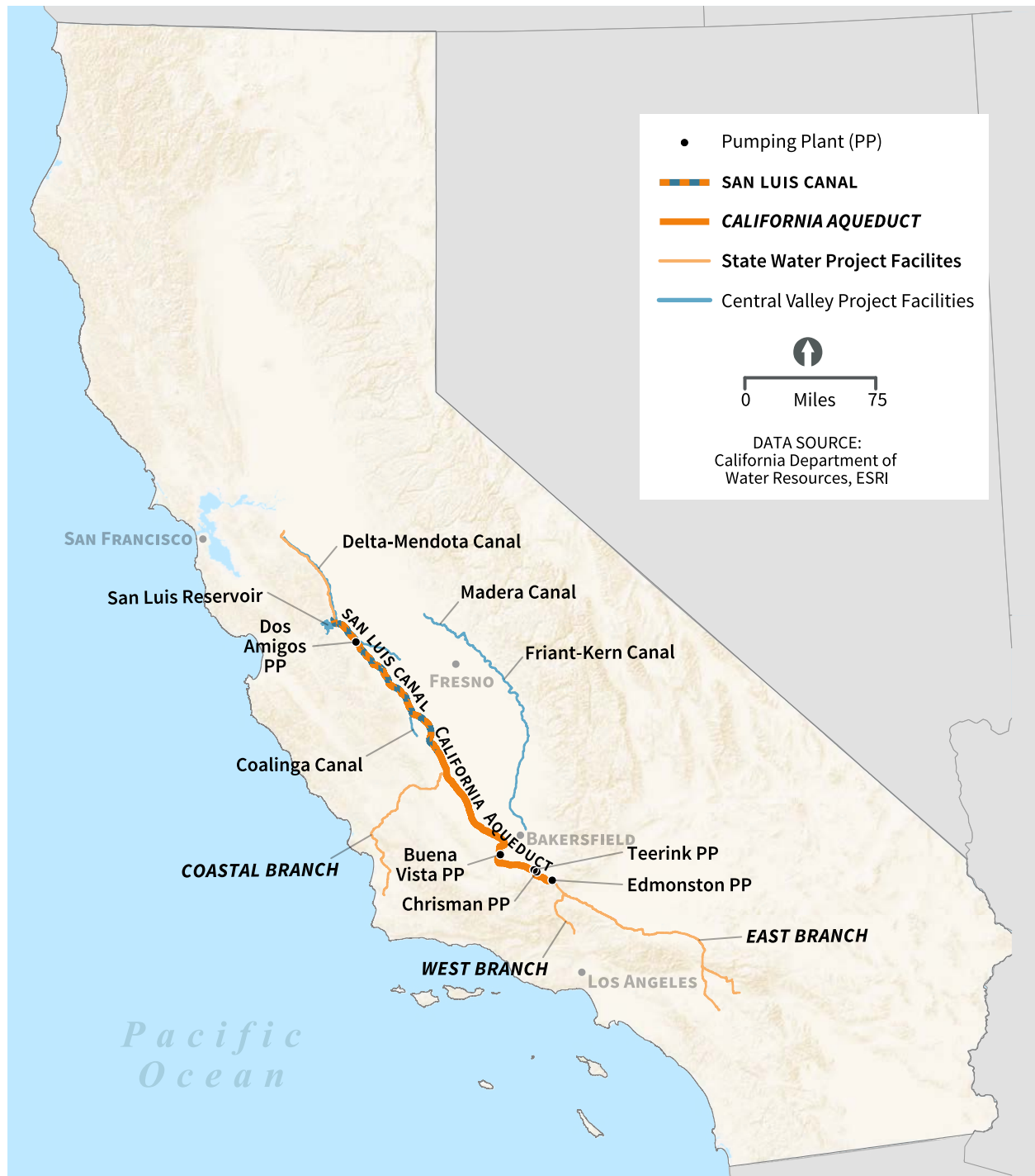
Figure 1. State Water Project and Central Valley Project facilities, with portions affected by subsidence shown in dashed blue and orange (San Luis Canal) and solid orange (California Aqueduct).
