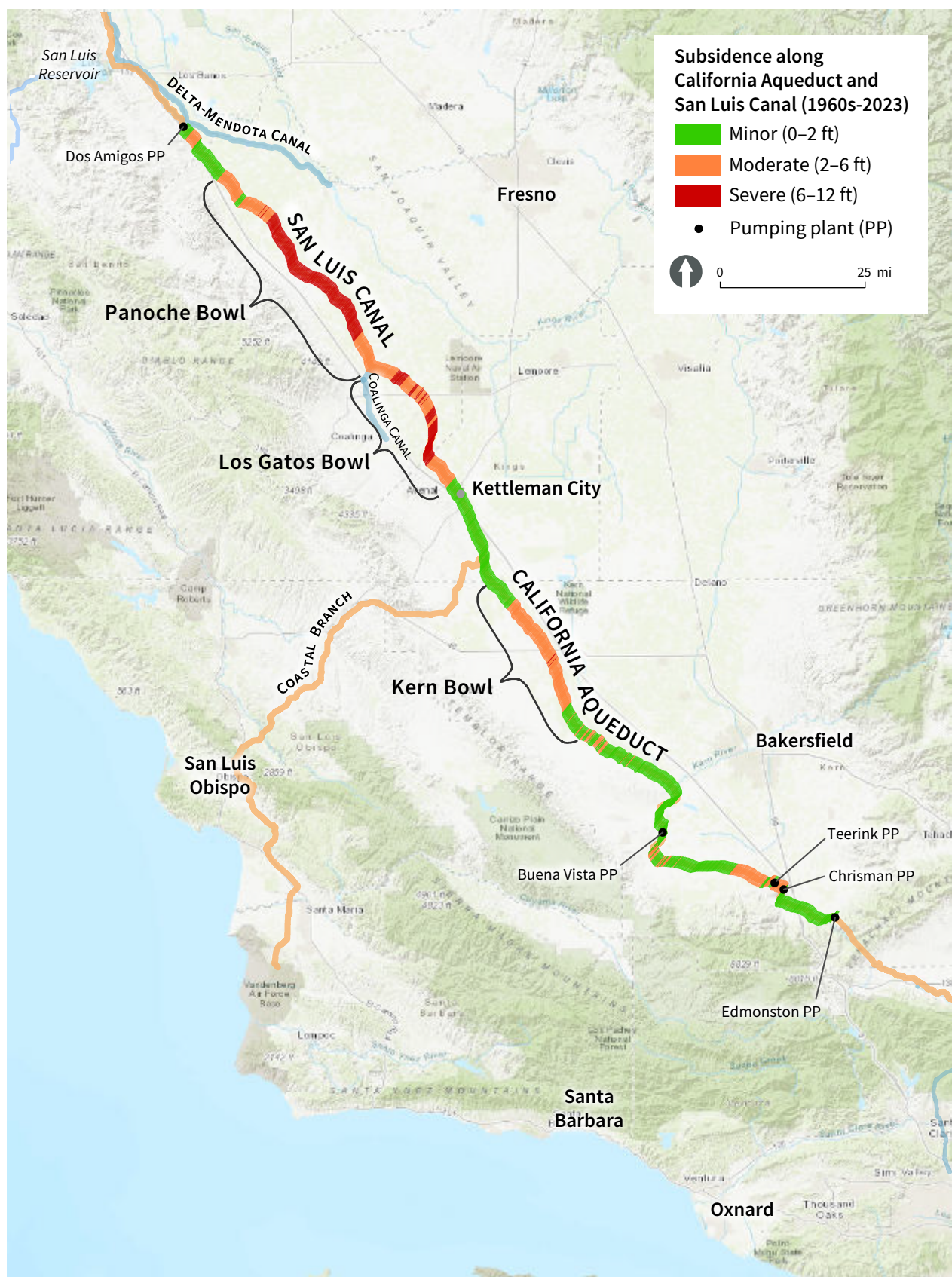
Figure 2. Subsidence along the San Luis Canal (a joint-use facility owned by Reclamation and managed by DWR) and the California Aqueduct (owned and managed by DWR).
