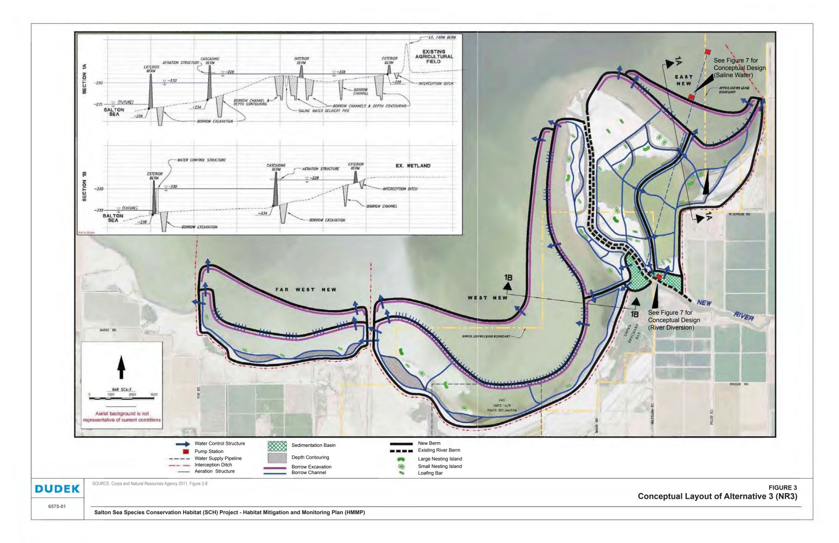
**Borrow Source.** The borrow source for berm material would be from excavated trenches along the exterior berm, shallow excavations, and borrow swales. The borrow swales would create deeper channels within an individual pond.
