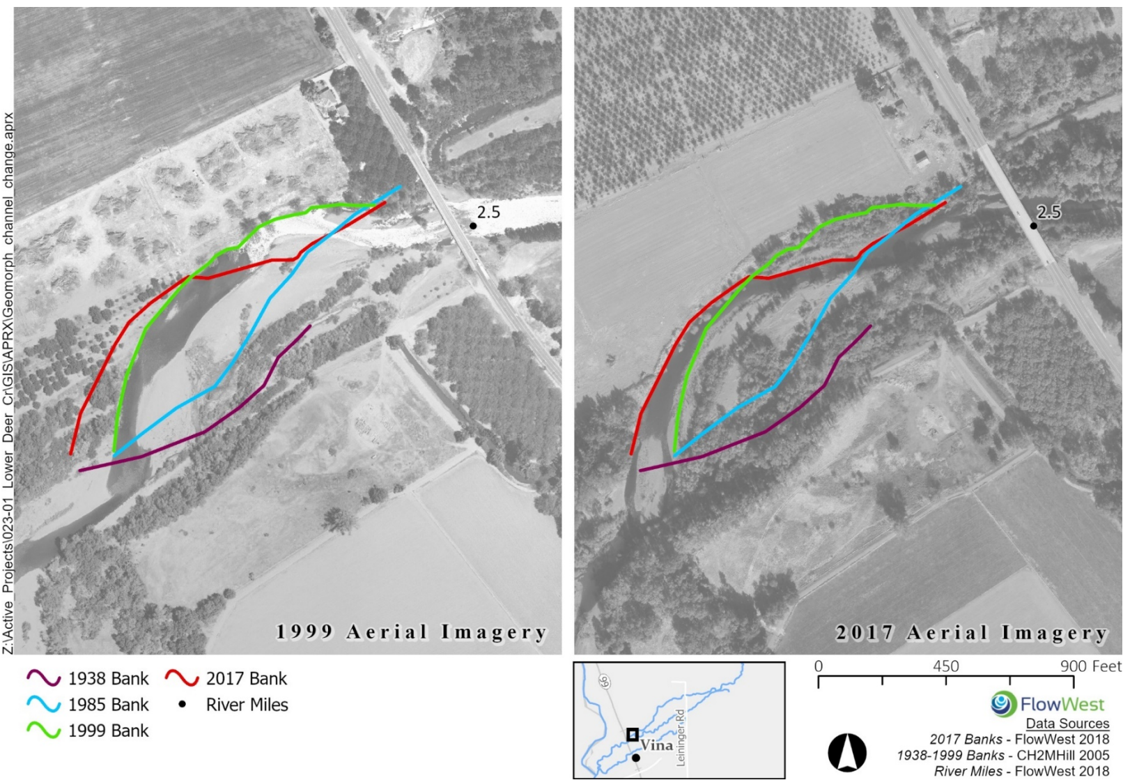
FIGURE 14: 1999 AND 2017 AERIAL IMAGES SHOWING THE CHANGE IN CHANNEL BANKS FOR THE IN-LEVEE REACH AT RM 2.5 FROM 1938 TO 2017.
