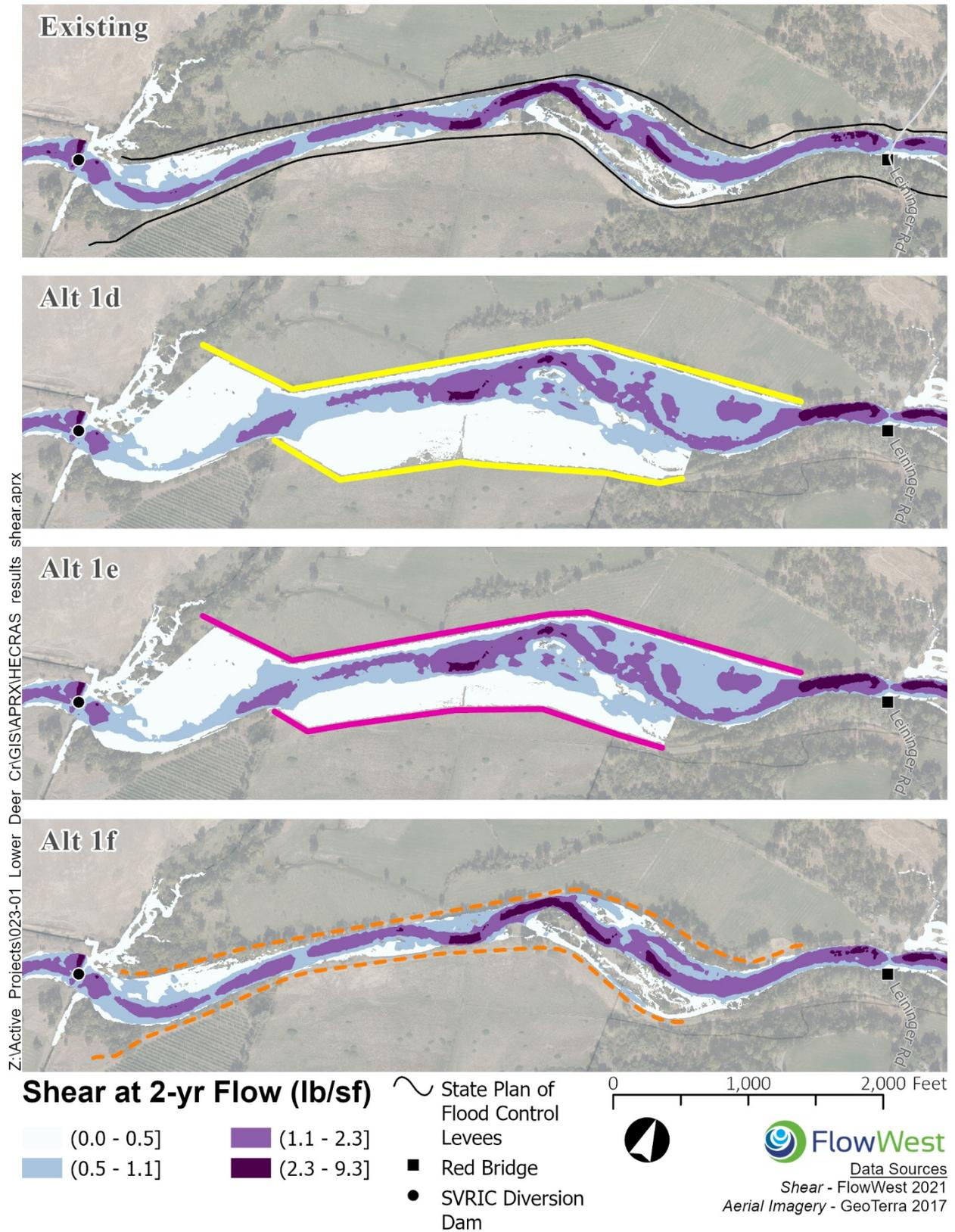
FIGURE 15: ALTERNATIVE 1A AND 2A SHEAR STRESS RESULTS AT 2-YR FLOW
