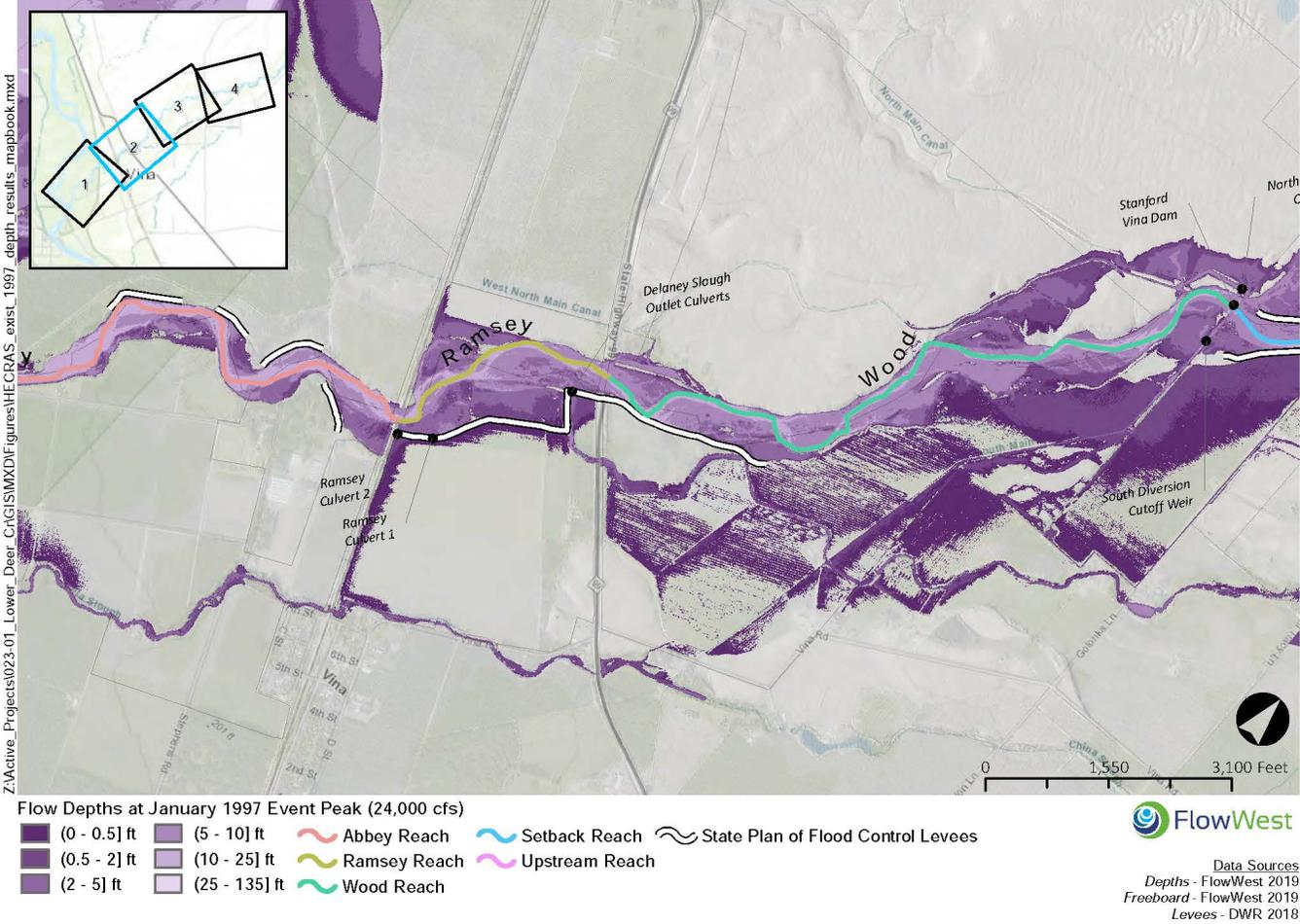
Figure B-2. Deer Creek Inundation Depth Map for Ramsey and Wood Reach
