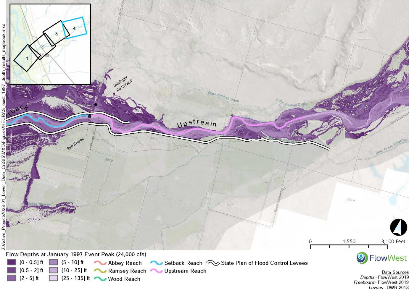
**Figure B-4. Deer Creek Inundation Depth Map for Upstream Reach**
