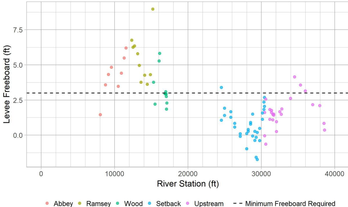
As with the DWR analysis, the 2D modeling evaluation indicated that a significant proportion of the project is out of compliance with the USACE O&M Manual. The reaches downstream of Highway 99E (Abbey and Ramsey reaches) were mostly found to be in compliance and reaches upstream of Highway 99E (Wood, Setback, and Upstream reaches) were found to be mostly out of compliance. The locations of project levees and freeboard evaluations are also mapped in Appendix A, Figures A-1 through A-4.
