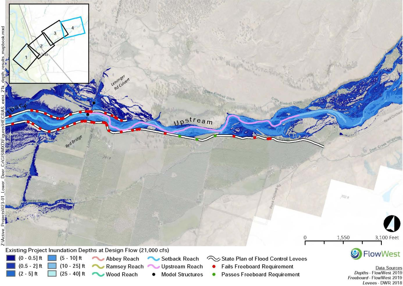
Figure A-4. Deer Creek Existing Inundation Depth Map for Upstream Reach
