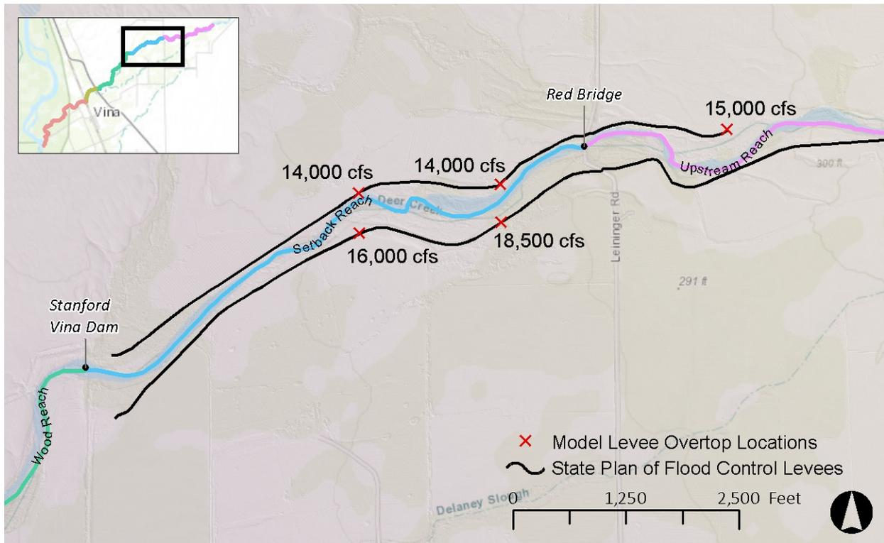
According to the O&M Manual for the Deer Creek Flood Control Project (Sacramento District Army Corps of Engineers, March 1957), the project has a design flow of 21,000 cfs. This corresponds to a near 50-year return interval flow event on Deer Creek. The project levees were designed to provide 3 feet of freeboard above the design flow water surface elevation profile. The O&M Manual requires freeboard be maintained throughout the life of the project.
