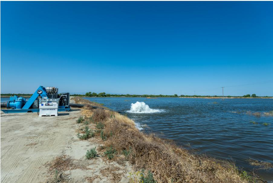
*DWR initiated an emergency program in the Central Valley to provide funding and rented equipment to local agencies to divert floodwaters for groundwater recharge. Here one of the rented pumps is being used by James Irrigation District (Fresno County) in May.*
