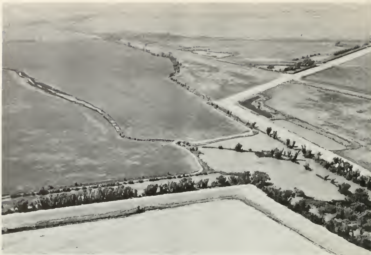
Two small meandering chonnels constitute the only outlet from the Knights Landing Ridge Cuf which is shown above entering the Yolo Bypass from the lower right corner of the photograph.
