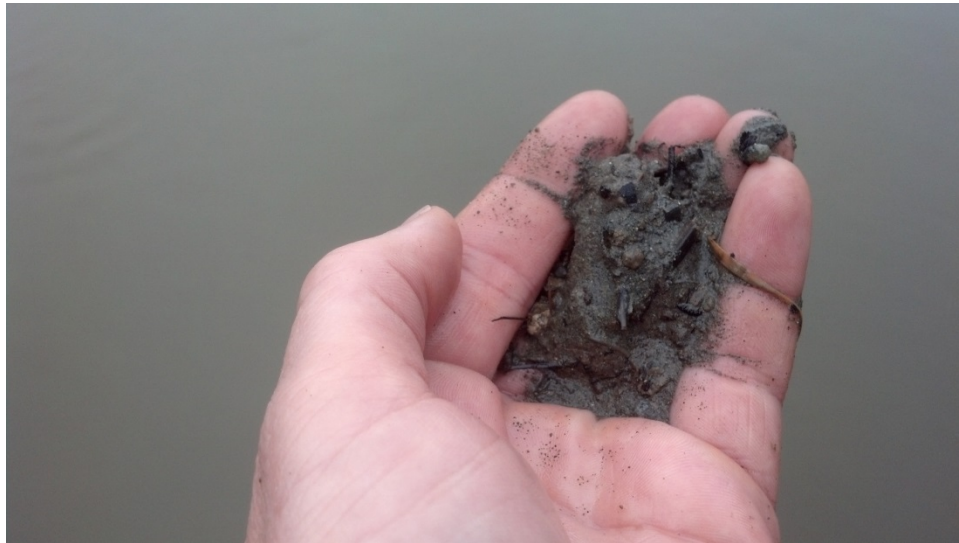
Figure 4.2.22. CBD channel bed material collected near the east bank illustrating silt to fine gravel composition.
