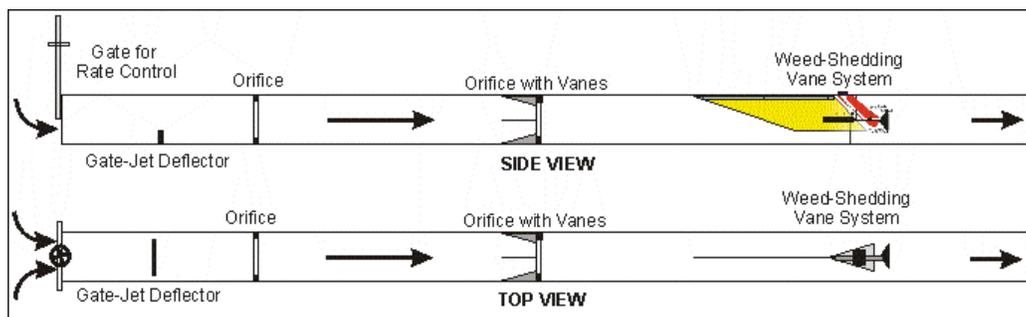
Figure 5. Flow conditioning vanes and weed vanes.
