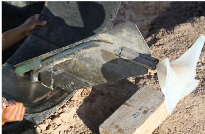
Figure 8. Propeller meter shows no weed fouling after a 24-hour run, using the propeller protection system, September 26-27, 2011.
