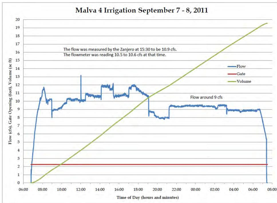
Figure 6. Record of irrigation delivery, September 7-8, 2011.
