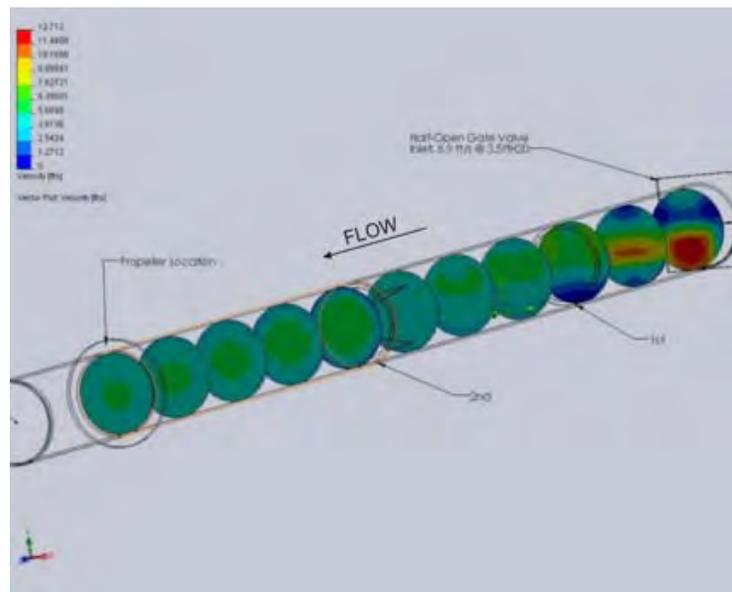
Figure 2. Results of Computational Fluid Dynamics Study.
