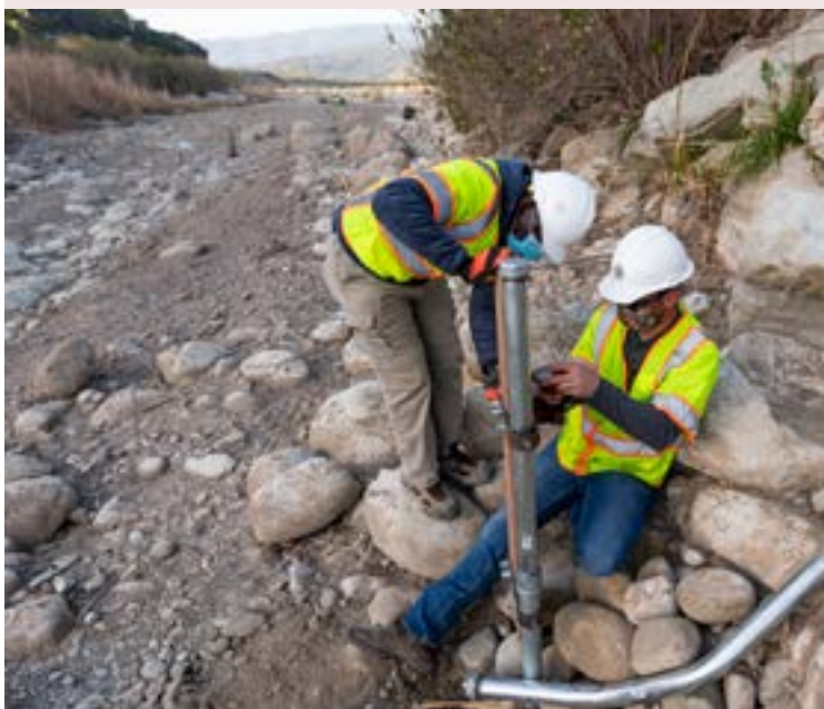
Working in a section of the Ventura River which routinely runs dry, Abiodun Aderonmu, a Senior Engineer with the Department of Water Resources, left, and DWR Engineer Technician Richard Holley, install a stream gauge that will be used to monitor and report the water level of the river in Ventura County. Photo taken April 8, 2021.
