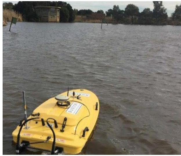
Figure 3. Example of Benthic Monitoring using a Teledyne Ocean Science Z-Boat. (AECOM and GHD, 2018)
