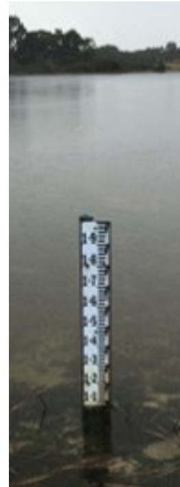
Figure 4. Example surface water stage (level) monitoring. (AECOM and GHD, 2018)
